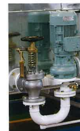
Mill pump ensuring comminution of any solid particles
