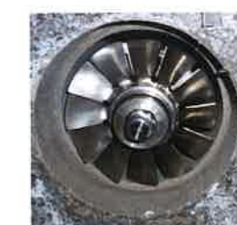
Maintenance free sludge burner of own design without any moving parts
